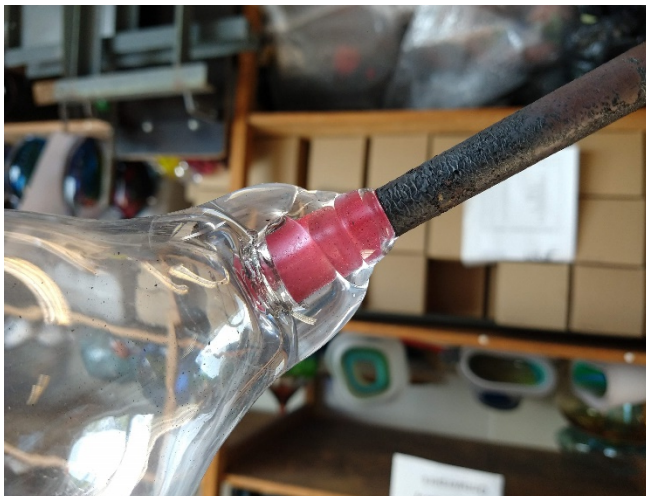
Figure 12. Photo of the reaction between copper and glass
